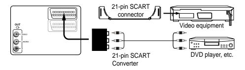
Note: If the equipment you want to connect is not equipped with 21-pin Scart, you can connect it by using the 21-pin Scart Convertor (supplied) as illustrated above.
